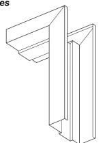
WELDED CORNERS Welded corners are tight fitting to provide a smooth seamless
