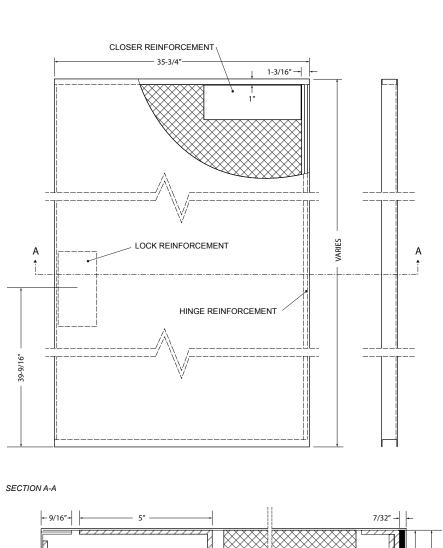
Door Construction Reinforcement Detail
